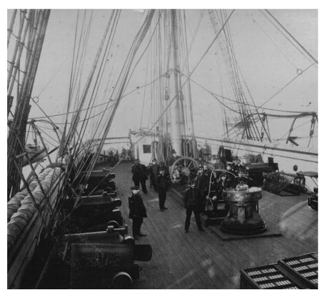
Figure 8 - Running rigging and shrouds "Hawser-Laid", right-handed.
